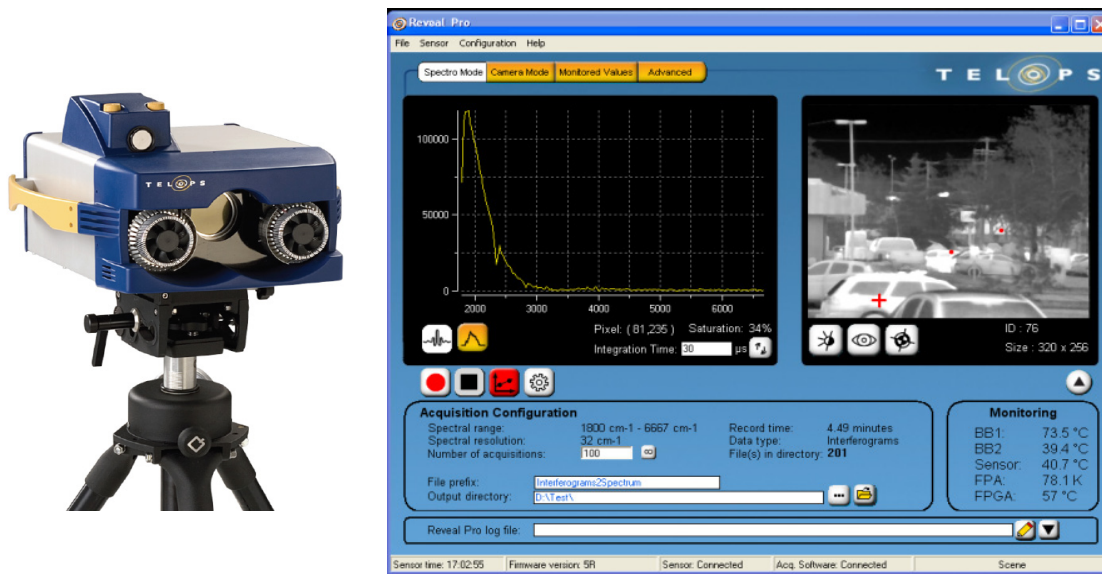
Fig. 1. Picture of the Hyper-Cam-MWE-Fast sensor (left) and screenshot of the Reveal Pro software (right) that gives the operator real-time feedback, including the broadband IR image and the spectrum of a selected pixel.
